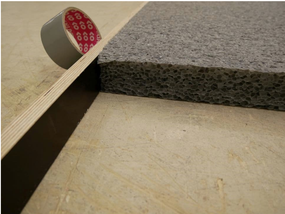
Figure B.4. Test set-up: Panels placed directly on the concrete floor, enclosing frame at lateral edges of the test set-up.
