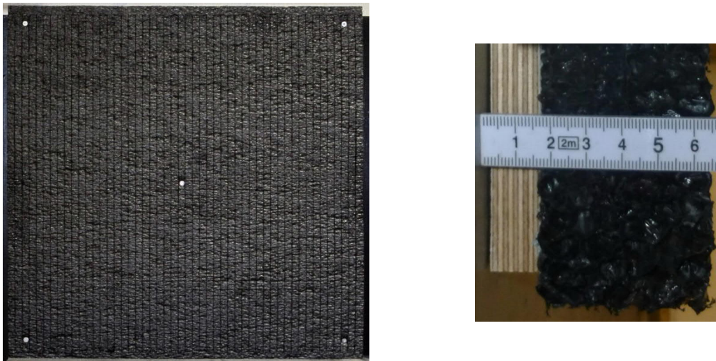
Fig. 1: Image of the set-up test body, consisting of a plywood panel (AW100) and the glued-on Whisper® NBO-40-A3 noise barrier plates, additionally screwed on.
