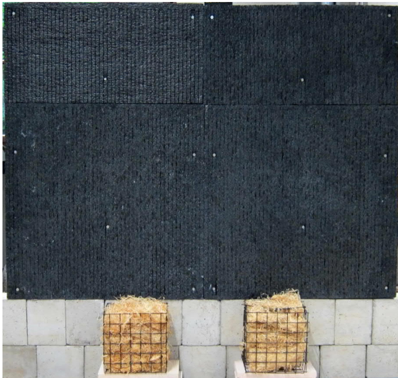
Fig. 1: Image of the set-up test body, consisting of a plywood panel (AW100) and the glued-on Whisper® NBO-40-A3 noise barrier plates, additionally screwed on.
