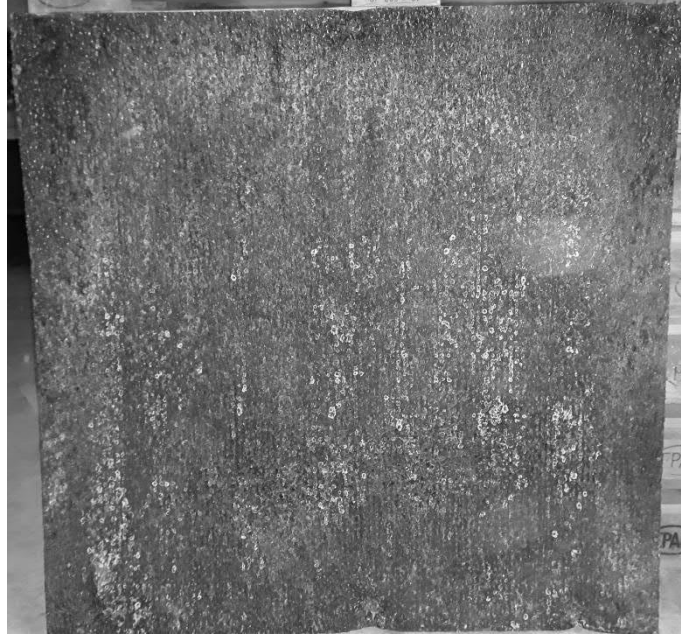
Fig. 12: Condition of the perforated Whisper® NBO-40-A3 absorber element after 30 theoretical years;
