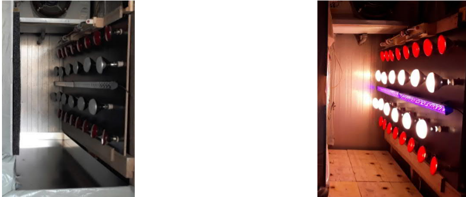
Fig. 4: View into the test chamber (left image) and onto the light panel in the switched-on condition (without collection pans and test elements; right image).
