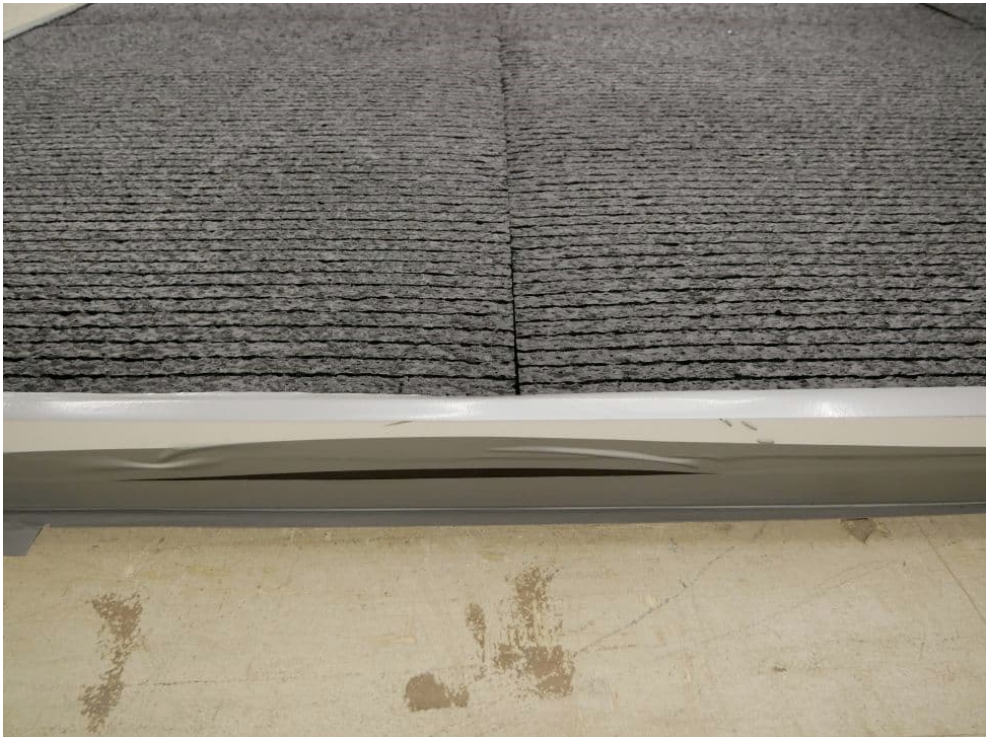
Figure B.5. Test set-up: joints to enclosing frame sealed with tape.
