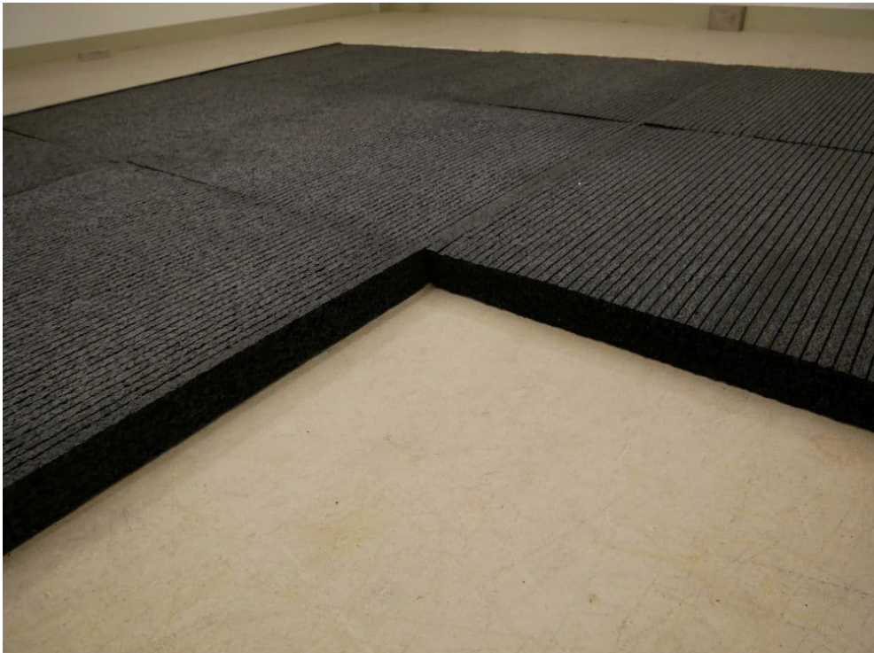
Figure B.3. Test set-up: Panels placed directly on the concrete floor, jointed bluntly.
